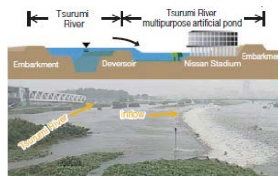
Inflow to retarding pond during flooding caused by Typhoon Phanfone
