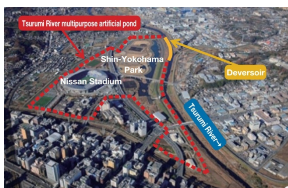
Photo 1: Areal view of the retarding basin
